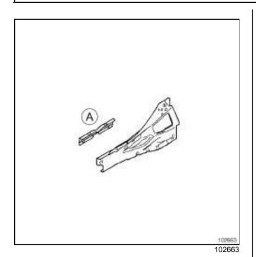
To replace this part, also order the sill panel rear reinforcement stiffener (A).
